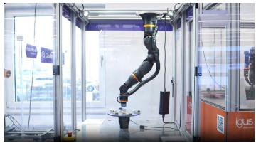
The system consists of a ReBeL 6-axis cobot mounted overhead in a Robocube cell. Cables are guided through a triflex cable carrier system for protection. The boards are located on a disc, under which there is a shaft gearbox used for the cobot's axes. Quality control is carried out by a camera system from SICK with a sensor for image analysis.
