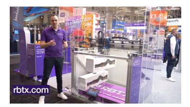
A typical palletizing application — often seen in the packaging industry — was demonstrated. The BLDC gantry was the right size to pick up standard Euro pallets in the work area and load them with ReBeL packaging for the showcase.
